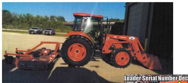
The tractor serial number decal is on the left frame, just above the front axle. The loader serial number decal is on the left loader upright but does not correspond to the tractor serial number, and must not be confused as a machine identifier. The image at right is of an M-7060 similar to the stolen tractor.
